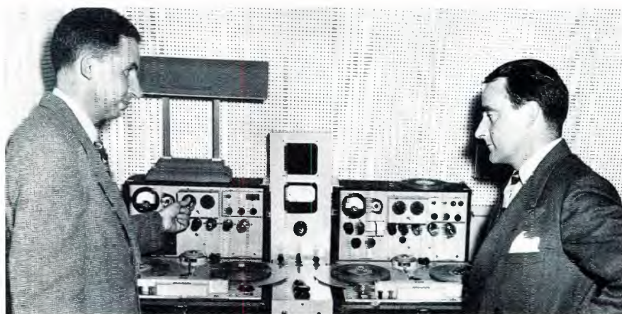
In this 1947 photo, engineer Mullin (left) shows his modified Magnetophon tape recorders to Murdo McKenzie, Bing Crosby's technical producer. Mullin's ability to edit on his high fidelity German recorders without generation loss created a sensation in American broadcasting. Mullin's machines later inspired the Ampex model 200.
