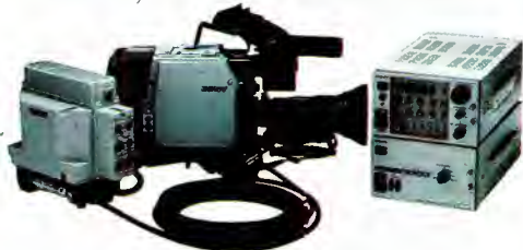
BVP-3, CA-30 Adapter, Digital Command Unit & 5,000' Triax to Camera Control.
