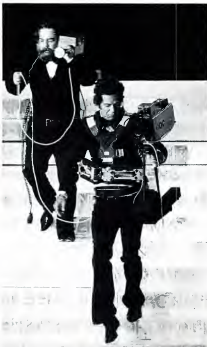
1978. On stage during the ABC-TV live telecast of the 50th Academy Awards presentation, operator Mayo Partee demonstrates the Oscar-winning Cinema Products STEADICAM system with NEC's MNC-71CP video camera, as Smokey DePetro follows him with portable microwave transmitter....an Academy Awards telecast first.
