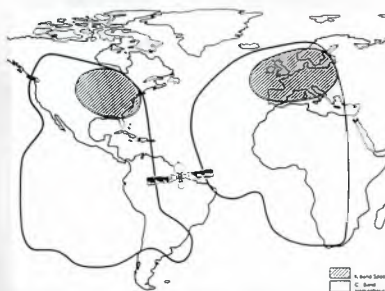
Figure 1. INTELSAT IBS C-Band coverage from 53° west longitude is shown by the unshaded circled areas on the map. Ku-Band spot beams, indicated by the striped areas, are steerable over a wide range that could include the West Coast of North America.
