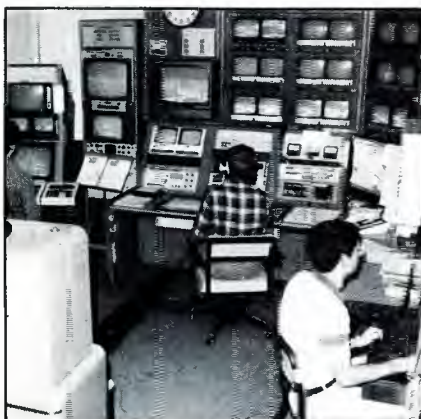
KTHI's master control room is shown as it is today. An American Data 3111 switcher is the heart of the system.
